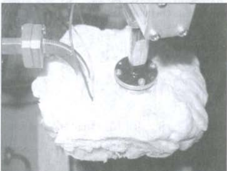
Liquid Nitrogen cooling: 1.5 dB NF/ 77K (4dB /290 K)
